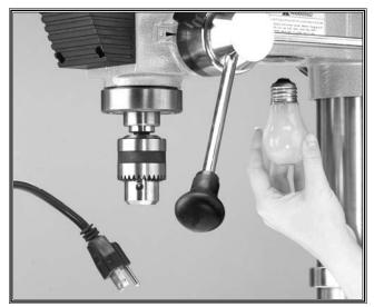
Figure 5. Unplug machine when changing bulbs.
